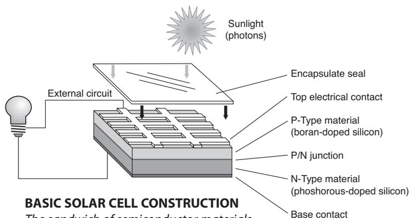
**BASIC SOLAR CELL CONSTRUCTION** *The sandwich of semiconductor materials produce electricity directly from the sunlight without any moving parts.*
